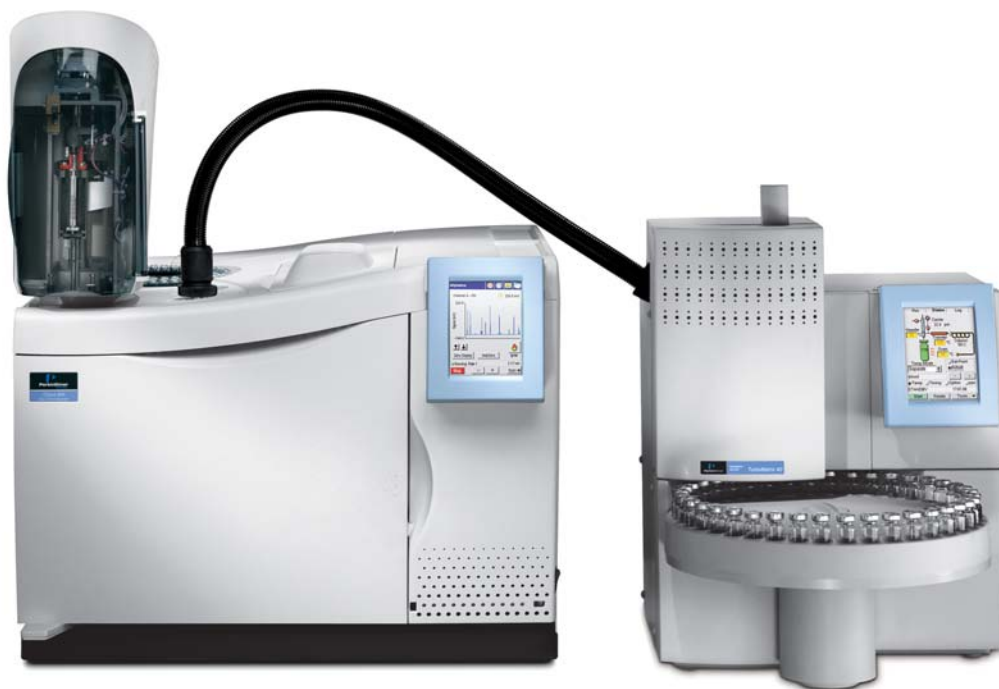
Figure 1. TurboMatrix Headspace 40 (right) with Clarus Gas Chromatograph (left).
