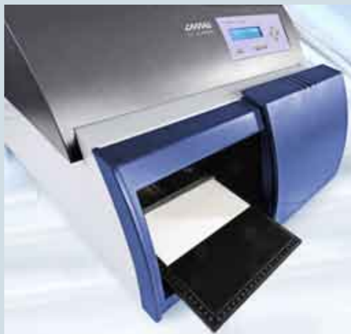
The object, here a 20x10 cm HPTLC plate, is positioned on the scanning table and simply inserted.
