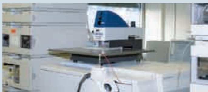
Hyphenation of TLC-MS Interface with mass spectrometer
