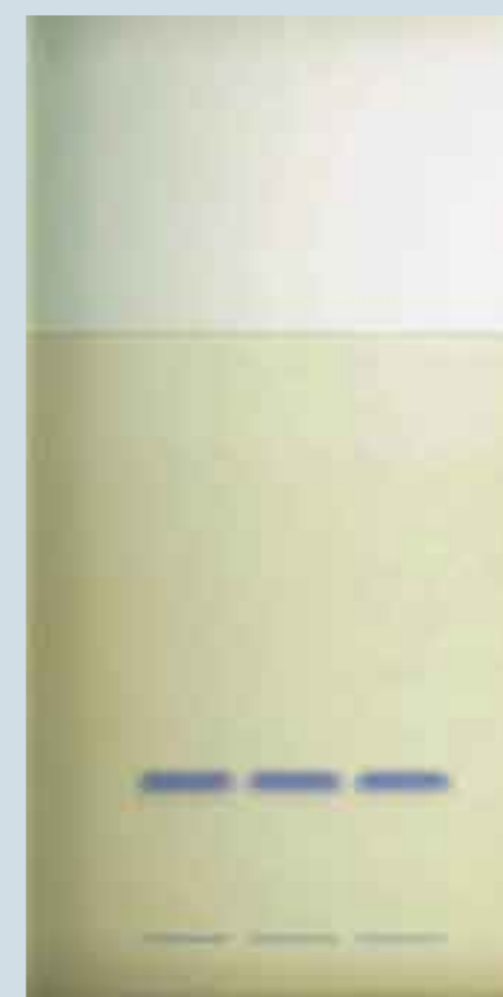
Derivatization of capsaicin with dichloroquinone-chloroimide-reagent / ammonia by spraying (1 g/L, left side) and by dipping (0.25 g/L, right side)
