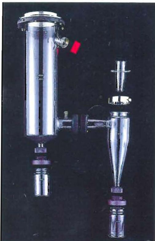
Suction filter at inlet
