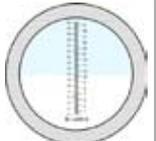
HR-140 Hand refractometer, 0-32% ATC, triple scale
