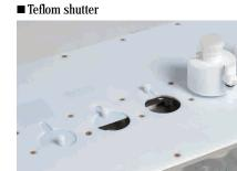
Teflon made shutter to protect aluminum block from dew
