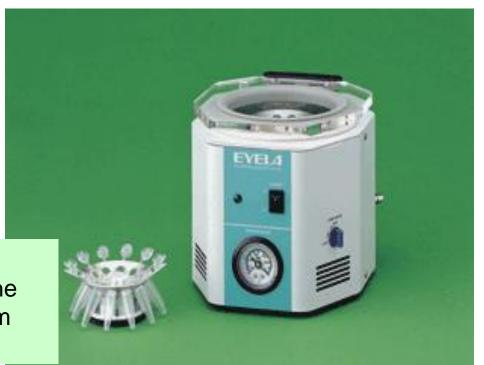
Common equipment for molecular biology. Mainly used for removing the solvents such as ethanol, chloroform from extracted DNA or RNA.
