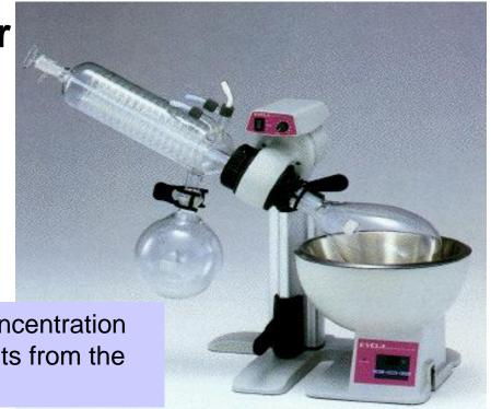
Widely used for the sample concentration mainly for removing the solvents from the extracted sample solution.
