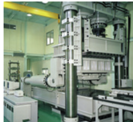
Shear load testing system for testing vibration-damping rubber
