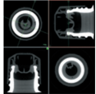
■ Internal observation of bottle caps The state of the sealing between a glass bottle and its resin cap can be checked by displaying any cross section desired. Also, gaps in the sealing and resin bubbles can be observed and measured using 3D display.
