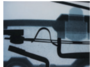
■ Fluoroscopic image of microswitch The state of microswitch contacts can be observed (e.g., for whiskers)
