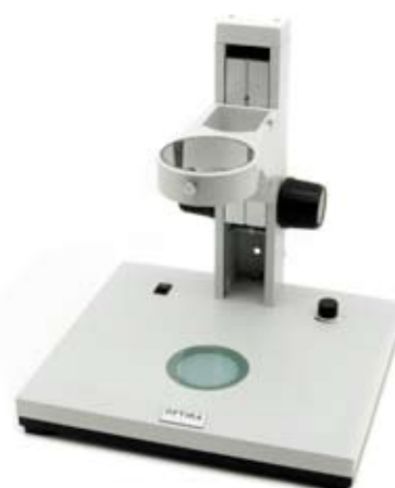
ST-153 Large plain stand with head holder and focusing mechanism. LED trans-illuminator with intensity control. Fixed arm type. Base: 320x280mm; fixed arm: 360mm.
