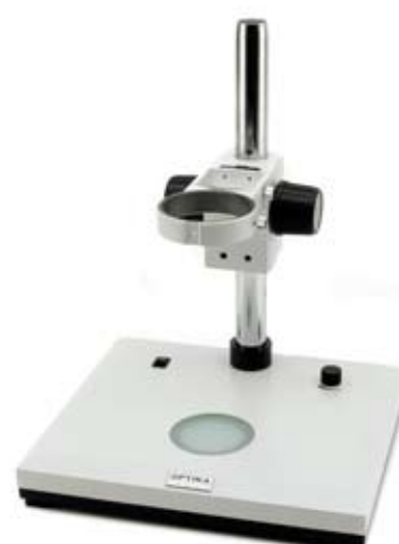
ST-151 Large plain stand with head holder and focusing mechanism. LED trans-illuminator with intensity control. Pillar type. Base: 320x280mm; pillar: \varnothing 32x360mm.
