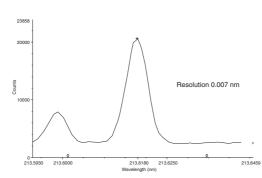
Figure 1b. 1 ppm Cu completely resolved from 1 ppm P at the 213.618 nm wavelength.
