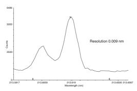
Figure 1a. 1 ppm Cu Interference on 1 ppm P at the 213.618 nm wavelength.
