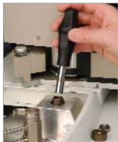
Place tool on liner cap. Align two pins on bottom of tool with two open slots on liner cap.
