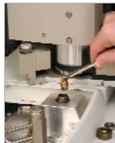
Use tweezers (cat. #20101) to remove liner cap.
