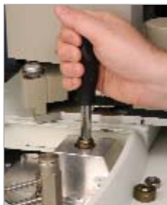
Turn counterclockwise to loosen liner cap.
