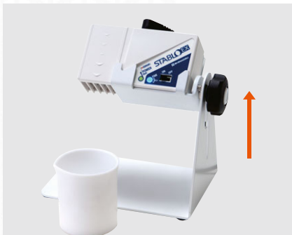
Quickly discharge container or bulk samples with fan ON.
