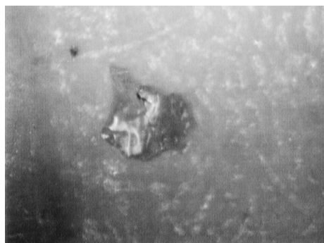
Fig. 7.6.1 Magnified photograph of the contaminant deposited on the paper
