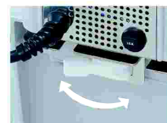
Bath can be easily dismantled by lever
