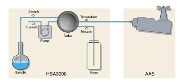
The analysis of samples with a high dissolved solids content has always been a problem in flame AAS. There is a strong tendency for salts to crystallize and cause blockages in the nebulizer or burner system. Historically, the only way to avoid this problem has been to dilute the sample until the concentration of dissolved salts is about 2% or less. This is a tedious and time consuming process.
