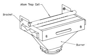
Figure 1: Diagram of the atom trap cell clamped onto its support bracket mounted on an air-acetylene burner.
