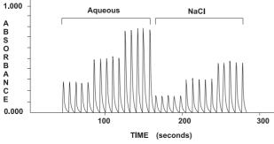
Figure 1: Comparison of 2,4 and 6 mg/mL Cu standards in aqueous solution and 10% m/V NaCl.
