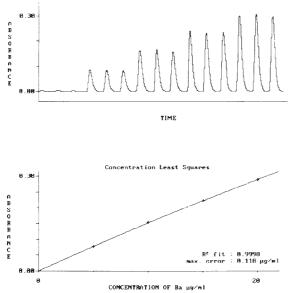
Figure 3: Standards traces and calibration curve for 5, 10, 15 and 20 µg/mL Ba in a 30% NaCl solution (peak height measurements).
