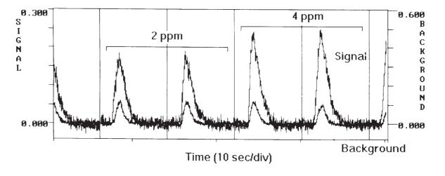
Figure 4: Signal and background traces for 2 and 4 µg/mL Fe in 10% m/V NaCl. Note different y-axis scales.
