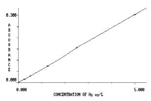
Figure 3: A representative calibration plot for mercury from  $0.25-5 \ \mu g/L$
