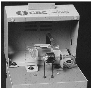
*Figure 6:* Detail of the MC3000 showing the inductively heated trap and the optical cell.
