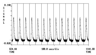
*Figure 4: Typical graphics traces illustrating 13 consecutive traces of mercury at 200 ng/L using a 100 second sample load time, with typical relative standard deviations of <0.5%*
