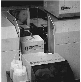
*Figure 5:* Installation of the mercury concentrator in a GBC 906 Elite AA, showing the HG3000 vapour generator, the MC3000 workhead and separate controller/power supply.
