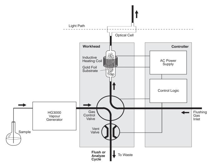
Figure 1: Mercury concentrator schematic.
