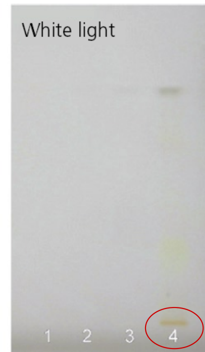
New yellow impurity caused color differences between batches of an API
