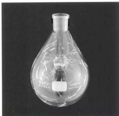
Breakage test of chemical coating flask
